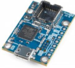
PureThermal 2 - FLIR Lepton Smart I/O Board
