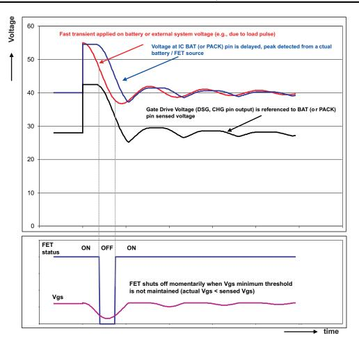
Figure 1. Transient Effect of FET Operation
