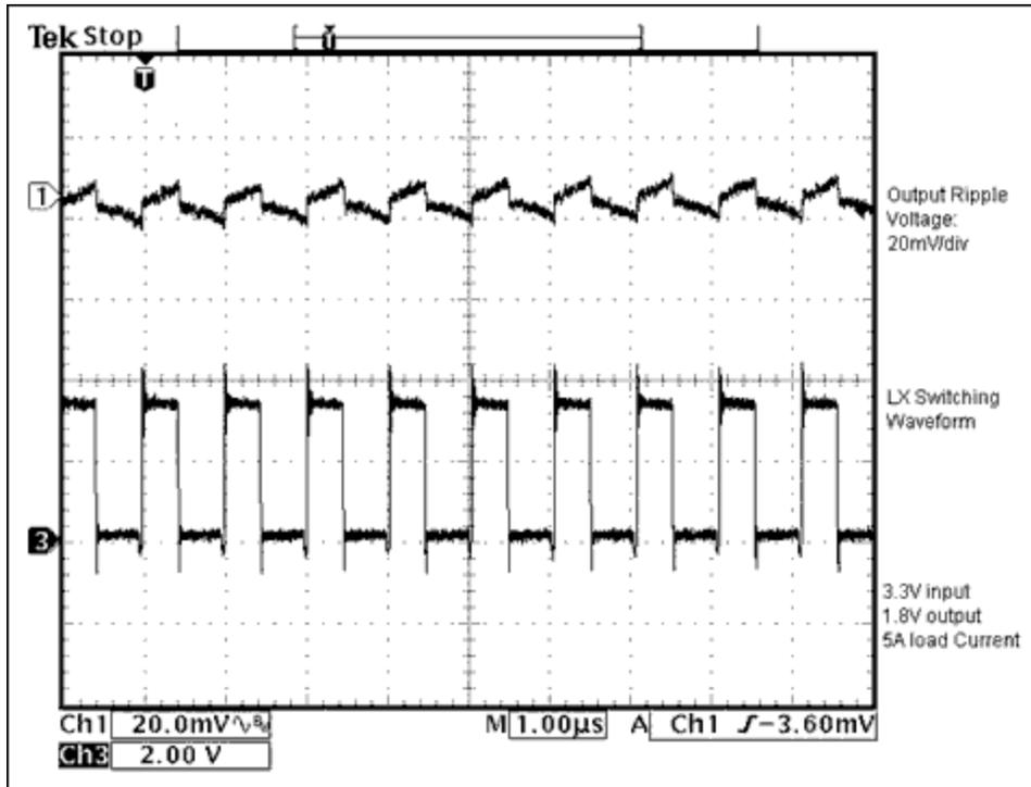
Figure 2. Output ripple voltage and LX switching waveforms.
