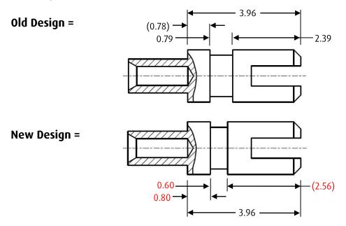
Existing stock will be to the old design. The new design will start being manufactured week commencing 18<sup>th</sup> Oct 2021, and will replace the old design as stocks are exhausted. The Technical Drawings and CAD Models are updated on the website.
