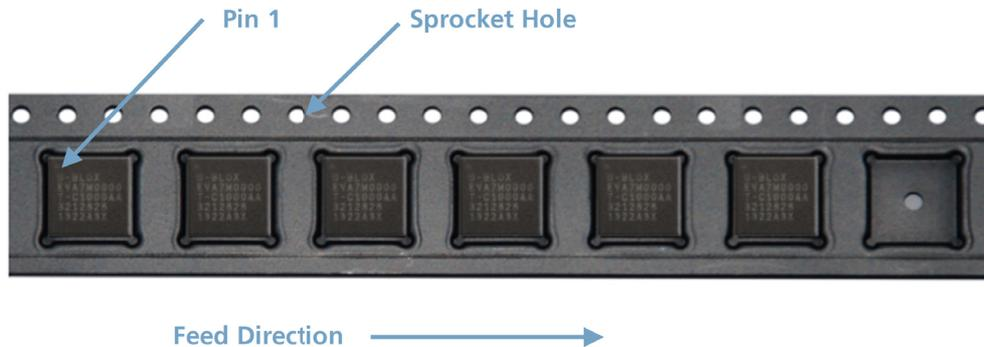
Figure 5: Orientation of EVA-7M modules on the tape
