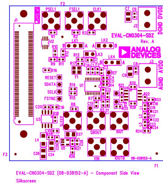
Figure 19. EVAL-CN0304-SDZ Component Side View Silkscreen
