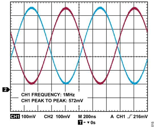
Figure 15. 1 MHz Output Signals on the IOUB and IOUBB Test Points
