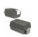
CDBA240-HF Comchip Technology DIODE SCHOTTKY 40V 2A DO214AC
